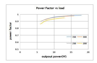
IT FIT 18 CS L Typical Power Factor vs. Load
